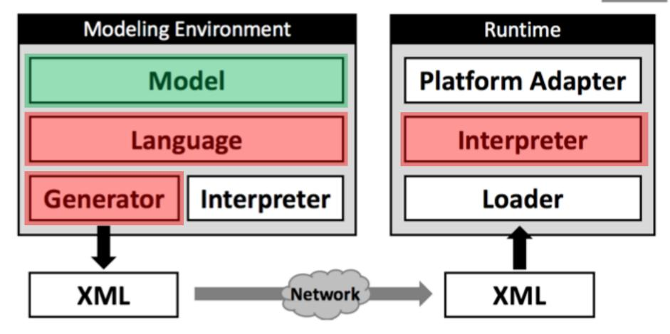
**Tools** may introduce additional systematic errors if faulty. Safety standards require reliable mitigation of such errors.
